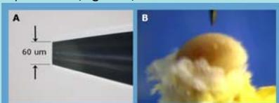
Figure 3: (A) Dimension of the indenter tip. (B) Indenter positioned perpendicular to the cartilage surface before starting the routine.
